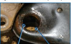
ENLARGED BALL JOINT RECEPTACLE IN LOWER CONTROL ARM, WHICH CAN CAUSE A LOOSE BALL JOINT FIT
