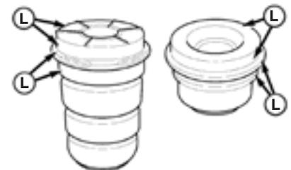
In the figure above, a smaller jounce bumper is used in the Pacifica and short-wheelbase minivans. A larger jounce bumper is used in the long-wheelbase models
