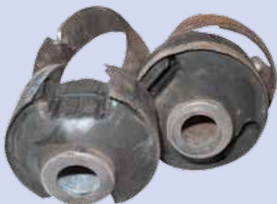
Metal outer ring separated from rubber bushing
