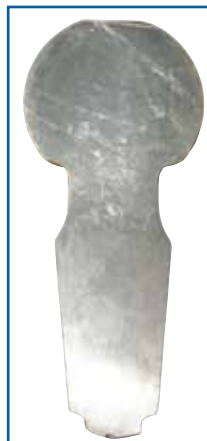
STUD WITH NO INDUCTION HARDENING IS 50% LOWER IN FATIGUE STRENGTH.
