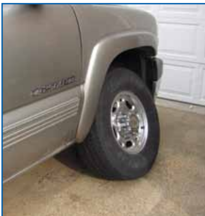
RESULT OF FAILED UPPER BALL JOINT
