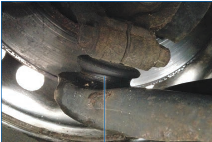
REPLACEABLE PART. REPLACE WITH MOOG® PROBLEM SOLVER® K500223 LOWER BALL JOINT.
