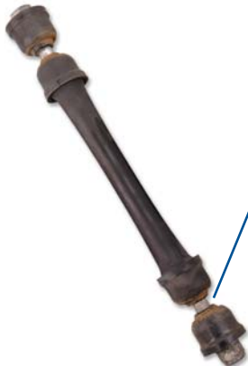
SMALL-DIAMETER OE BOLT Subject to corrosion and early failure
