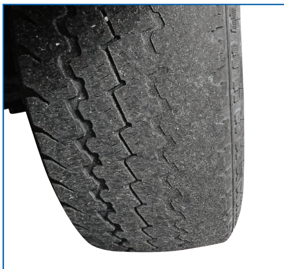
TYPICAL TIRE WEAR FROM EXCESSIVE CAMBER
