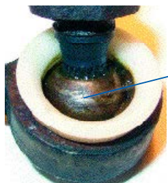
A FAILED FIRST OE DESIGN PART MEASURED 0.024" OF PLAY, A RESULT OF THE CORRODED STUD WEARING INTO THE BEARING SURFACE.
