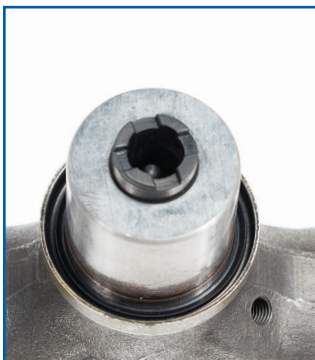
SUPPLIER 1: NON-INTEGRATED ANTI-DRAINBACK VALVE; NO THRUST WASHER
