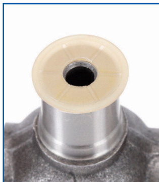
SUPPLIER 2: THRUST WASHER INCLUDED, BUT NO ANTI-DRAINBACK VALVE
