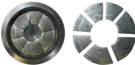
A disassembled failed OE part reveals a shattered spring
