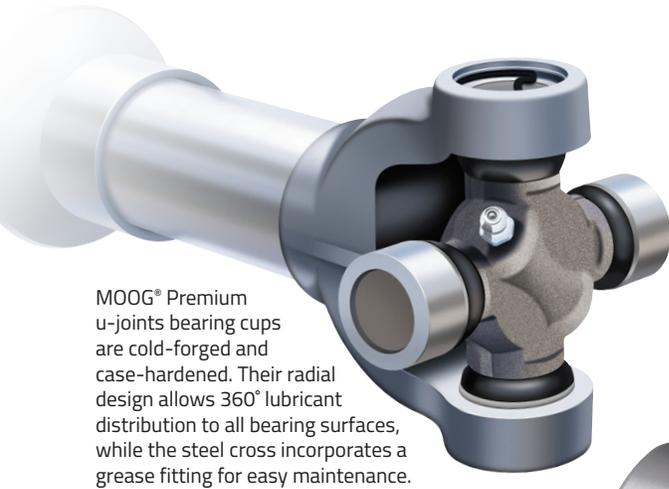
MOOG® Premium u-joints bearing cups are cold-forged and case-hardened. Their radial design allows 360° lubricant distribution to all bearing surfaces, while the steel cross incorporates a grease fitting for easy maintenance.
