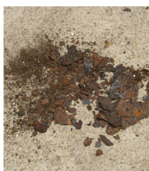
Note: It's imperative to remove loose rust to prevent an excessive air gap.
