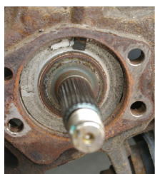
Knuckle with hub removed
