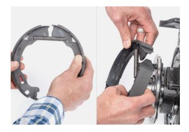
Step 3 – Using the front shoe and the parking brake boss' leverage, rotate the front shoe onto the knuckle.
