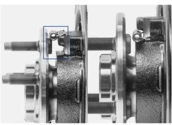
**Incorrect Due to Interference**This is due to the interference between the lug bolt and the parking brake boss.
