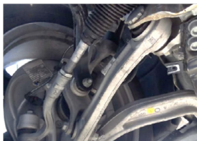
Tightened track control arm bushings with 'hanging' wheels (figure A)
