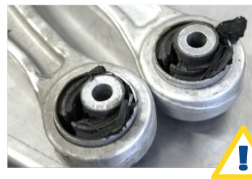
Premature wear of the track control arm bushes.
