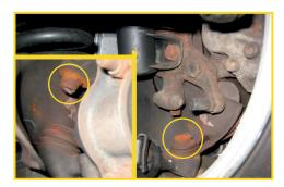
A fatigue failure of a ball pin neck can cause a driver to lose control of the vehicle. The combination of an induction hardened ball pin neck and MOOG's patented carbon fibre bearing not only enhances both the performance and the service life of the ball joint but also improves driver safety.
